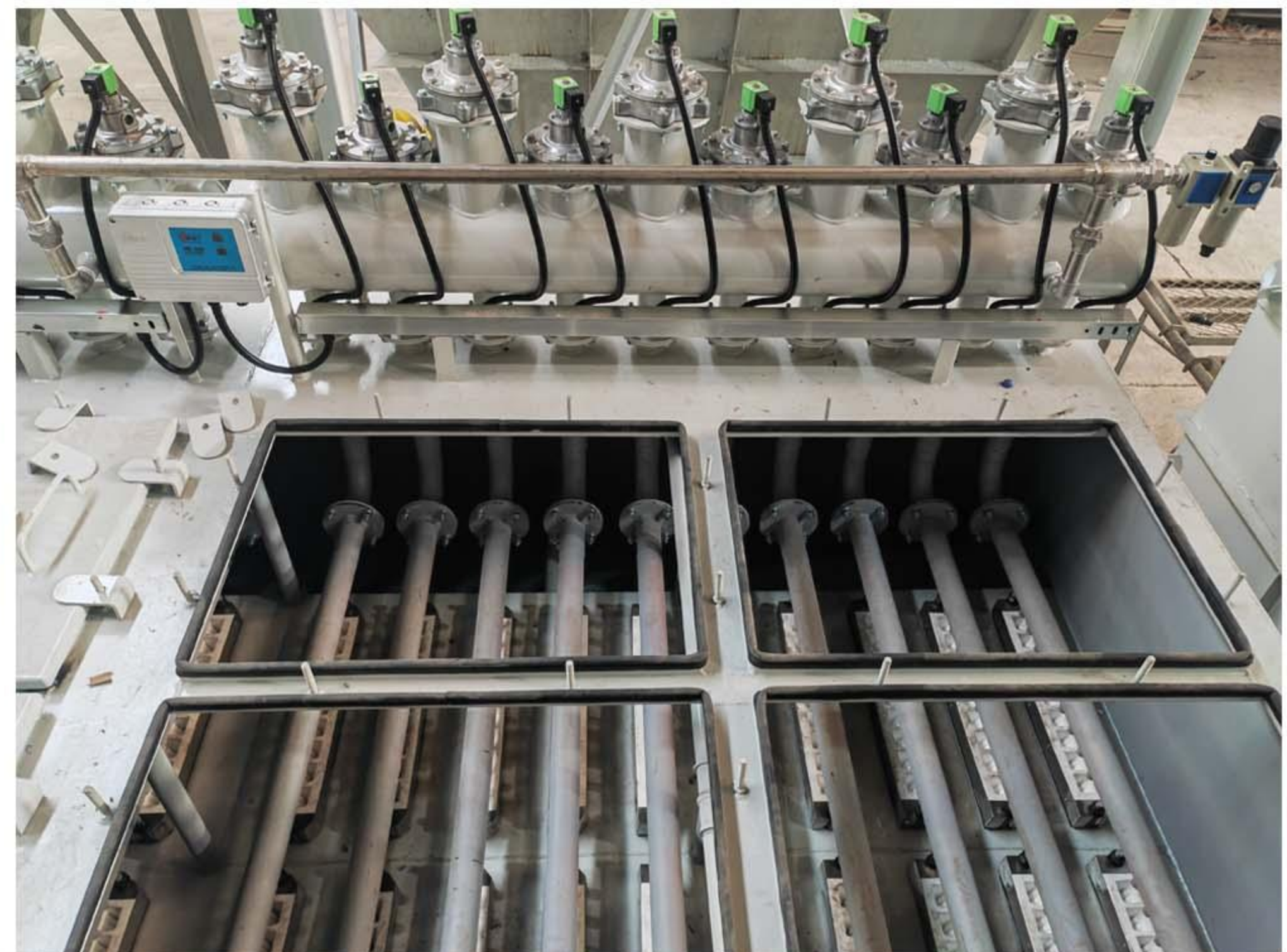
Top-Mounted PE Sintered Plate Installation Diagram
