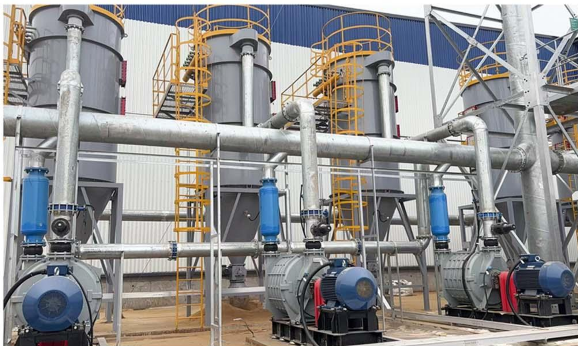
Vacuum Cleaning Dust Collection System for Crystal Pulling Workshop, Photovoltaic Module Plant - Baotou
