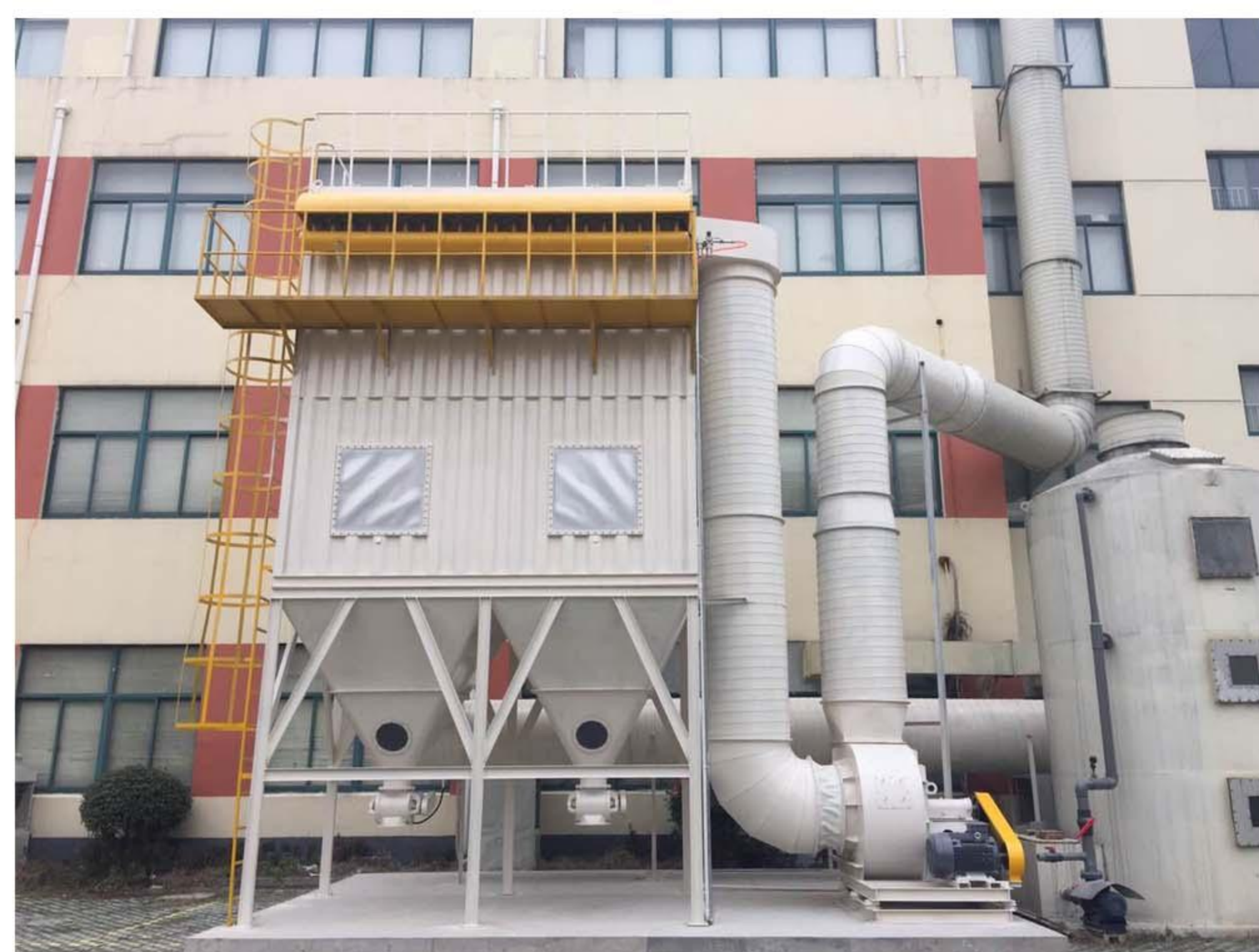
Dust Collection System for Computer OEM Grinding Process - Suzhou
