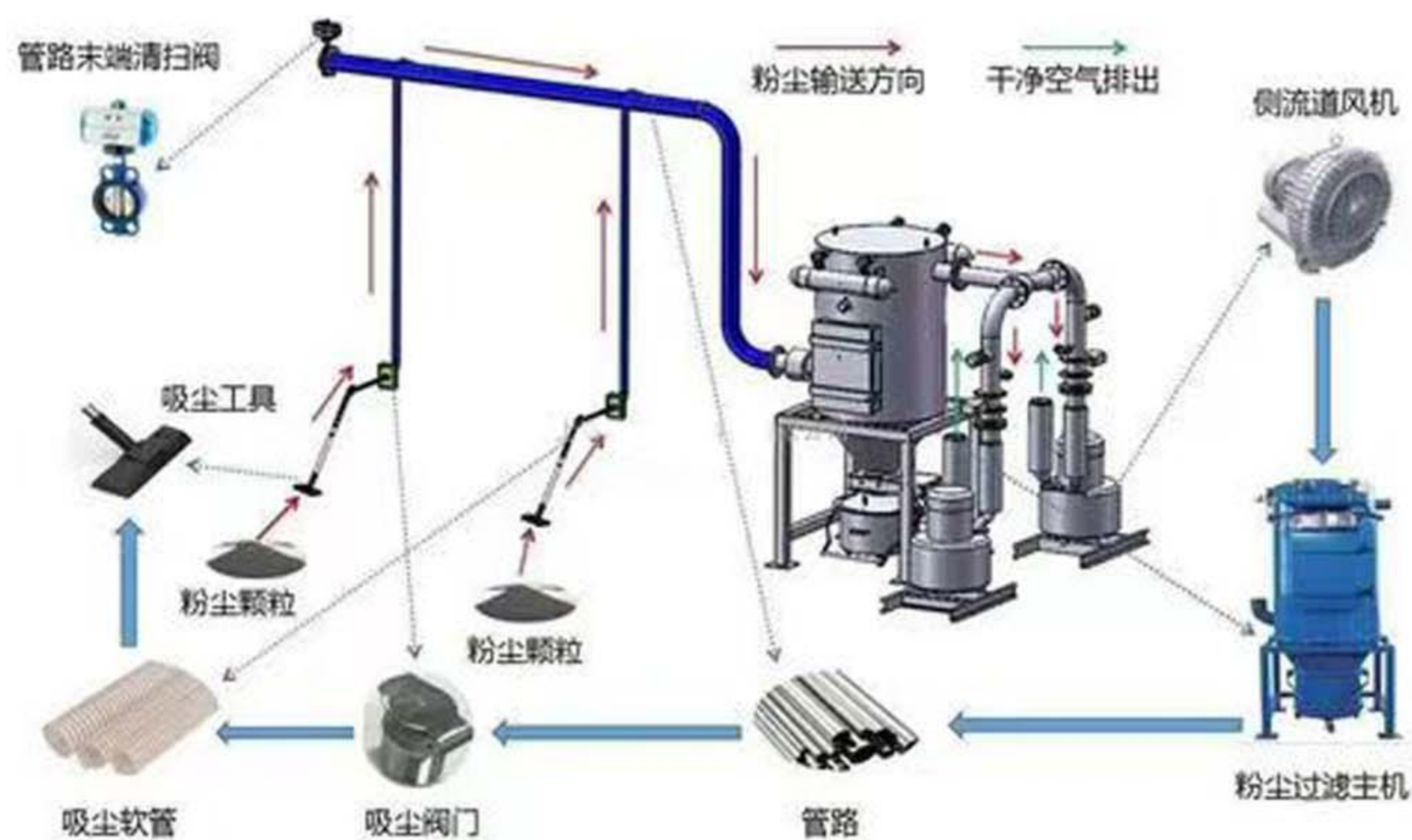
Vacuum Cleaning Process Flow Diagram
