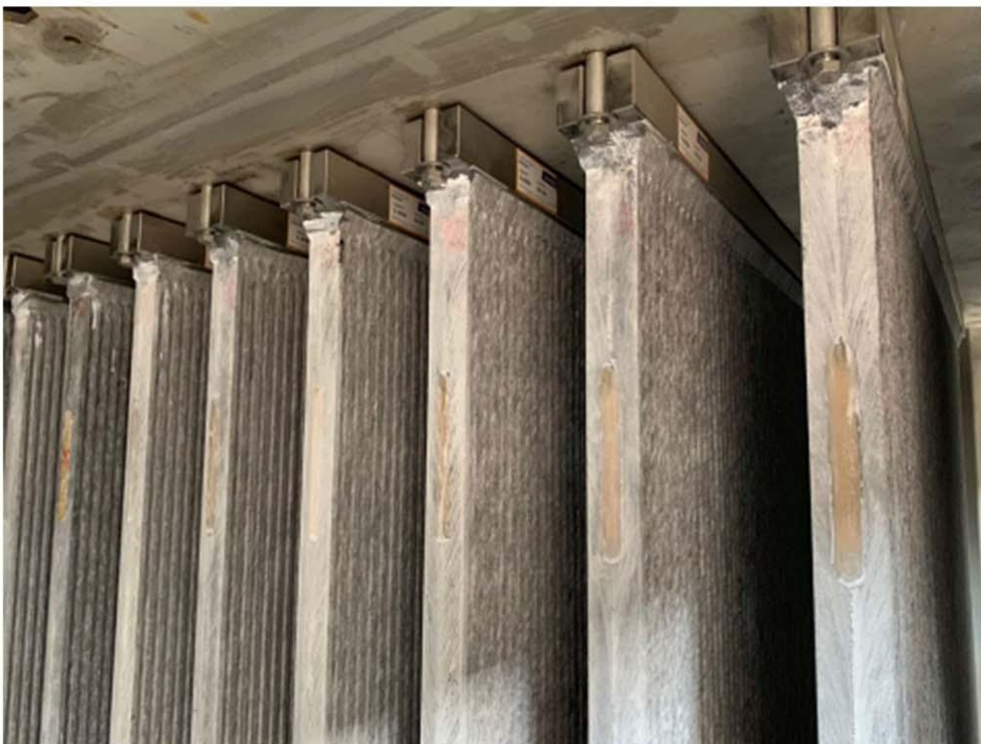
Bottom-Mounted PE Sintered Plate Installation Diagram
