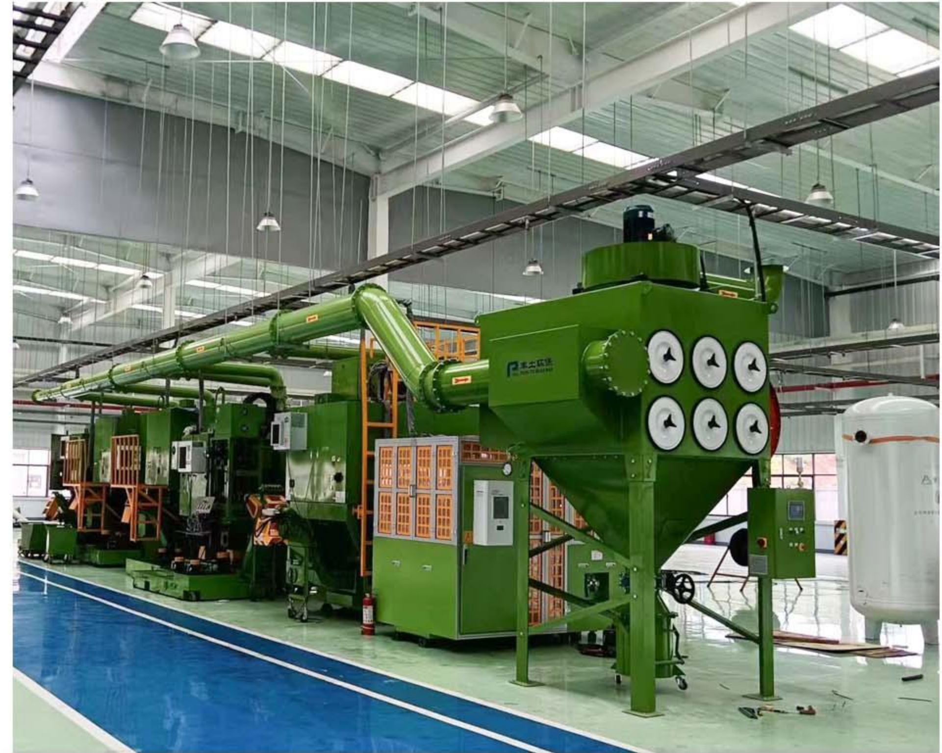
CNC Machining Dust Collection Ducting Example Image (Q235B Carbon Steel)
