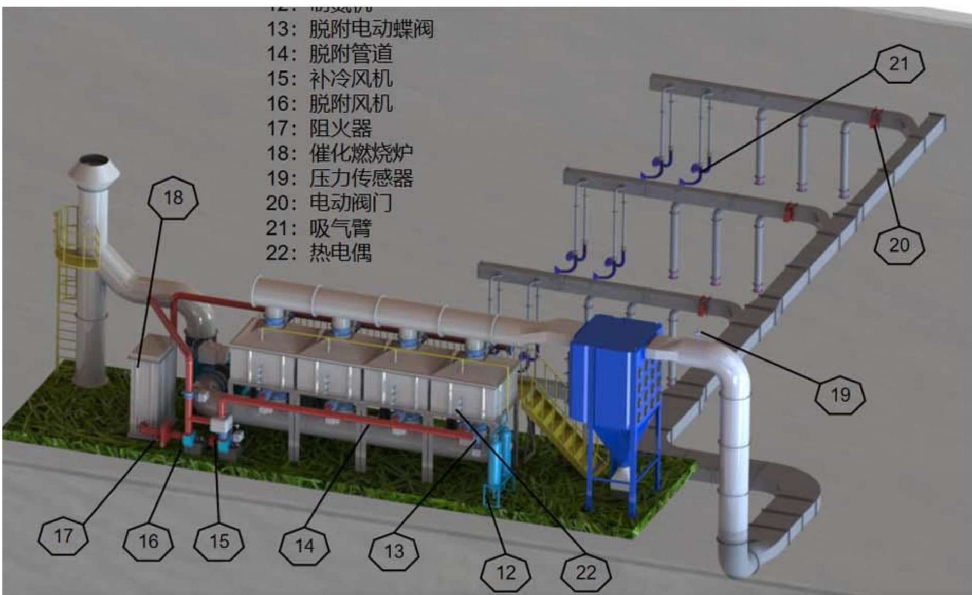
Process Flow Diagram of Adsorption - Desorption RCO System
